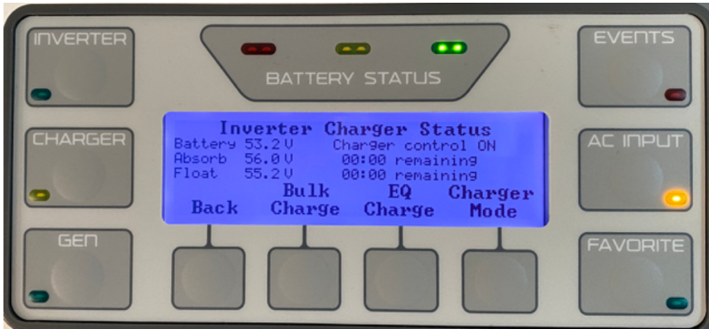
Figure 6. Mate3 display. This shows the controls for accessing the off grid configuration information. This screen indicates normal operation. Press Charger button on left to get this display.
